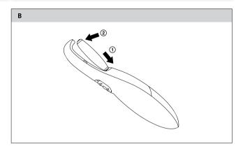
To remove, press the abrasion roller A@ down towards the handle A® and remove it
