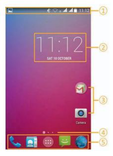
**Information panel** with information about current notices of applications can be viewed by pressing and pulling the status line downward. Tapping on an item opens the associated application, swiping to the side removes the notification from the list. The top right corner of the information panel contains an icon for removing all displayed notifications and also for switching to the usual settings quick access menu.
